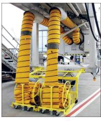
Tapered Adapters also insert directly into the duct system for the final connection to the aircraft connecter. ITW GSE Adapters are available in two styles - straight tapered or 90° tapered.
