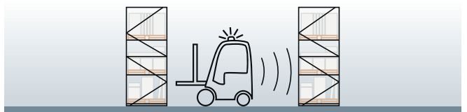
Anti-collision with stationary objects such as shelves, vehicles or other obstacles
