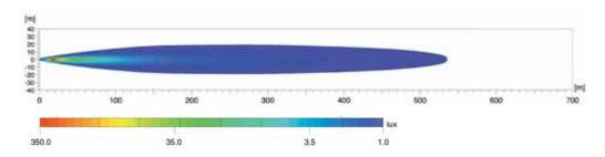
The light distibution shows 2 high-beam headlamps each in function.
