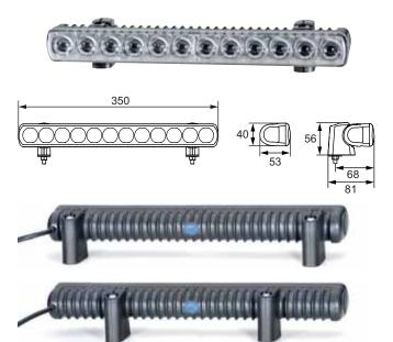
The variable positioning of the two plastic brackets using the clamping joint on the housing ribs allows flexible mounting options on the vehicle.
